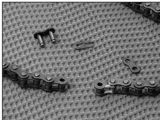
Figure 47. Chain removed from table by removing the master link.
